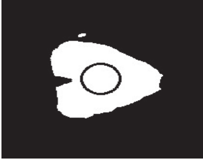
Fig. 7. This figure illustrates the initialization of inflating balloons in an arc-off frame. This is a binary image by thresholding the original frame. The black circle inside the white region represents the initial position of the inflating balloons.
